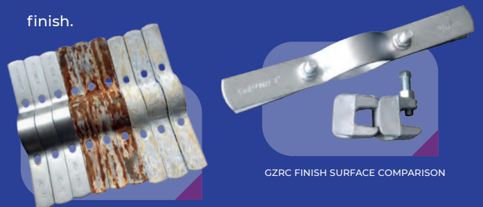
GZRC FINISH SURFACE COMPARISON AFTER 240h OF 20% NATURAL SALT SPRAY TEST
